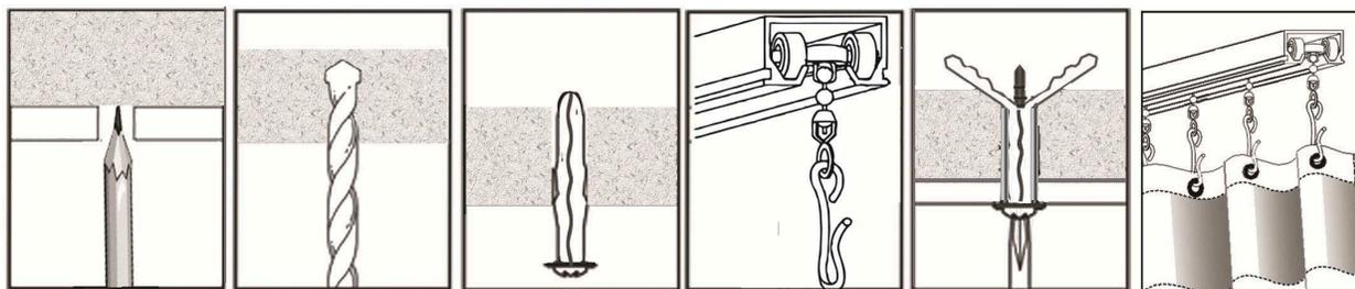
Using the Track as Pattern, Mark Holes on Ceiling    Drill 1/8" Pilot Hole in Drywall, If No Stud, Drill 1/4" Hole    Insert Drywall Anchors in Dry-wall if No Stud    Insert in Track same # of Carriers as Grommets    Attach Track to Ceiling at Mounting Holes    Hang Shower Curtain and Enjoy Your New Trax
